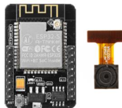
Fig c. This figure shows the module of ESP32 camera.
